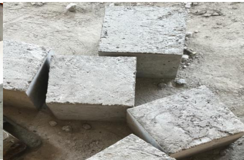
Fig. 2 Cubes with 2%NS and 1%NA
